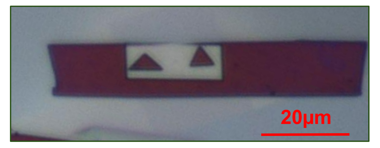
Figure 11: Optical image of sub-wavelength wedge samples fabricated through mechanical exfoliation and FIB etching
