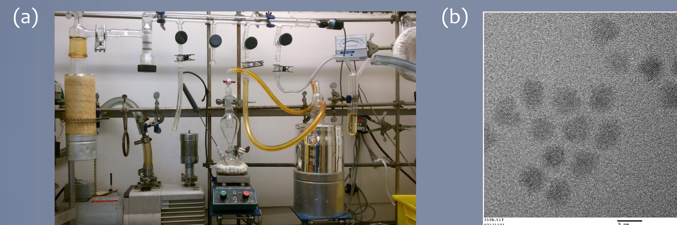
(a) Typical synthesis setup using Schlenk line. (b) High resolution TEM of CdSe nanocrystals. Preferential growth was performed following a modified version [2]:
