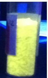
Yttrium aluminum garnet (YAG) doped with cerium Ce) fluoresces when irradiated by photons
