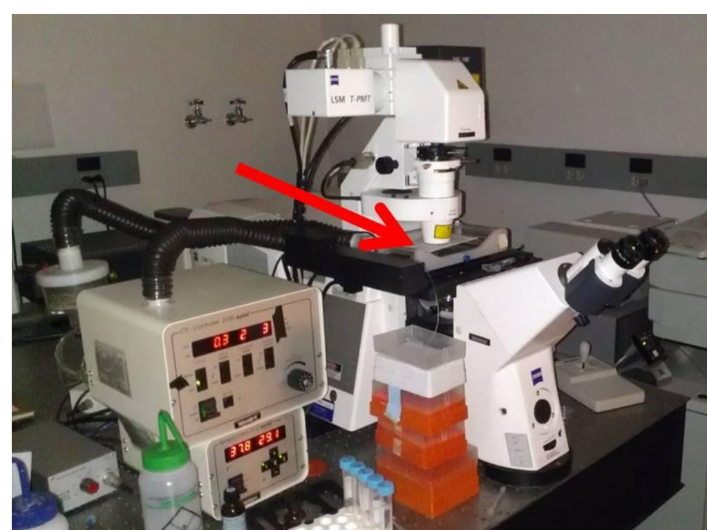
Figure 4: Confocal microscope. Arrow indicates where microfluidic device is placed.
