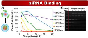
Polymers successfully bind siRNA and form NMPs. A) Electrophoretic mobility shift assays demonstrate that NMP formation depends heavily on N:P ratio - the molar ratio of cationic DMAEMA repeats to anionic phosphate charges on siRNA. B) aligned gel images.
