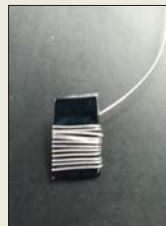
Wire mask applied to Al 2 O 3 /Si wafer
