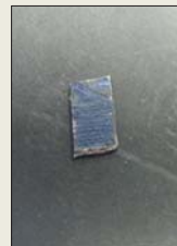
Wafer after deposition (Au @ 4.6 V/cm for 26 min, GraphenX @ 105 V/cm for 45 min)
