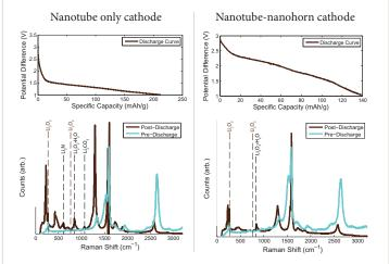
The non-ideal discharge curves, low specific capacity and complicated post-discharge Raman spectrographs without Li2O2 peaks suggest that significant side reactions are occurring during discharge. This may be due to apparatus leakage, electrolyte contamination, or the effects of the TOAB remaining from functionalization.
