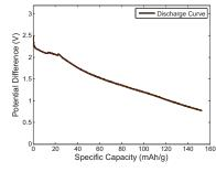
However, batteries made using these unfunctionalized CNT cathodes display a similarly non-ideal discharge curve and low specific capacity (see discharge curve right). This suggests that the primary contamination causing secondary reactions that hinder battery performance is not from the TOAB used in functionalizing the CNTs.
