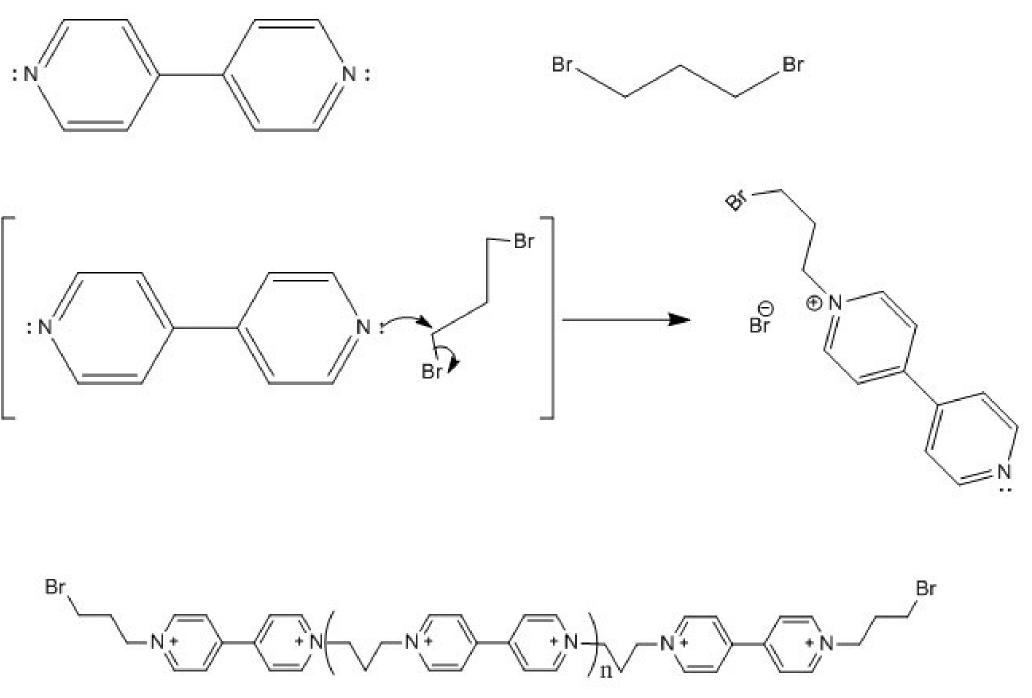
Reaction utilizes the Menshutkin mechanism and converts a tertiary amine to a quaternary ammonium salt. Monomers (4,4'-bipyridine and p-dibromoxylene or throughout reaction.
