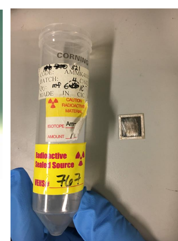
Figure 8: Americium-241 Alpha Particle Source
