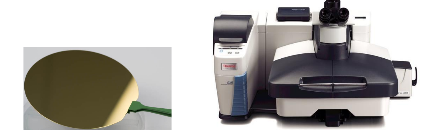
(Left) Gold coated silicon wafer. (Right) Thermo Scientific DXR Raman microscope
