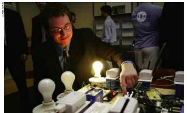
Corey Toomey and his team's "smart home" device, which can remotely control a home's lights, appliances, and heating and air conditioning via the Internet or a cell phone
