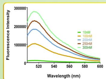
Spectral overlay of standard F5M solutions for calibration
