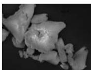
Created YAG:Ce phosphor through combustion synthesis
