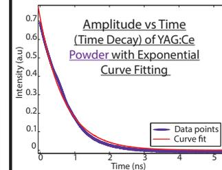
Lifetime of the phosphor is determined from the equation of the exponential curve fit
