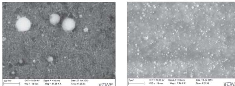
Nanoparticles have an average size of 100-200 nm and a consistent spherical shape
