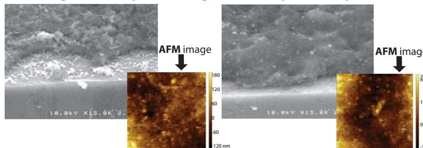
Film created by evaporation onto silicon substrate. Film is approximately 500-700 nm thick.
