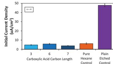
Though the 6-carbon functioned best of the acids, it did not outperform the hexane control. Overall, all of the monolayer-treated samples greatly underperformed plain etched Si; possibly an adverse effect of the monolayer deposition process.
