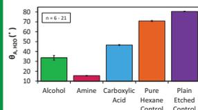
The contact angle for a water droplet on Si indicates the wettability of the surface, confirming the presence of organic monolayers.
