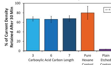
Over time, however, it appears that the organic monolayers provide a significant increase in stability: likely due to protection from Si surface oxidation. Chain length, on the other hand, does not seem to make a difference in the first 30 minutes.
