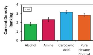
Photochronamperometry was used to measure the current through the PSI film under red light. The highest current density, at 50  $\mu\text{A}/\text{cm}^2$ , was achieved using the carboxylic acid monolayer.
