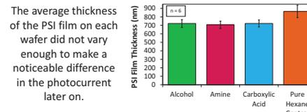
The average thickness of the PSI film on each wafer did not vary enough to make a noticeable difference in the photocurrent later on.
