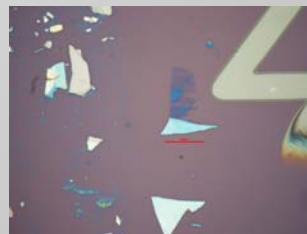
Fig. 3a. Single layer MoS 2 under 100X microscope. The scale bar is 20 \mu m.
