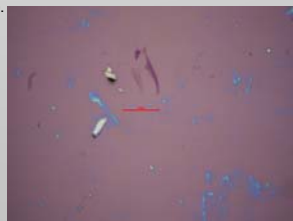
Fig. 1a. Single layer graphene under 100X microscope. The scale bar is 20 \mu m.
