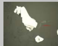
Fig. 4a. Single layer graphene on glass coated with PMMA under 100X microscope.
