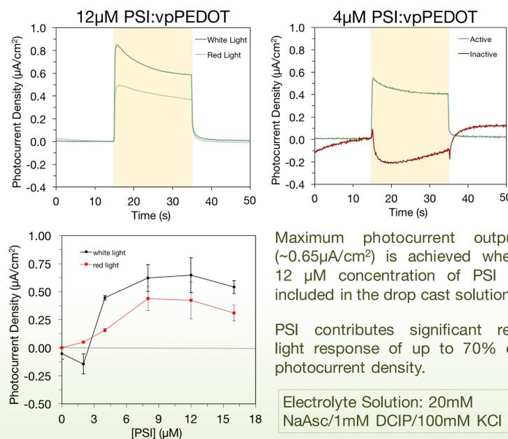
Maximum photocurrent output (~0.65µA/cm²) is achieved when 12 µM concentration of PSI is included in the drop cast solution.
