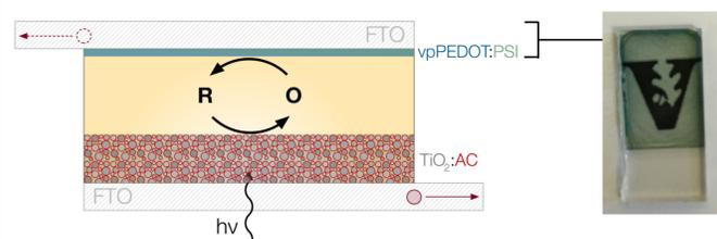
vpPEDOT:PSI is proposed as an alternative to platinum at the counter electrode of dye sensitized solar cells (DSSCs), where PSI allows for the reduction of ions in the mediator solution, reducing resistance to charge transfer.
