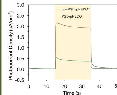
Preliminary results show a ~4x increase in photocurrent density upon the addition of plasmonic nanoparticles in the drop cast solution.
