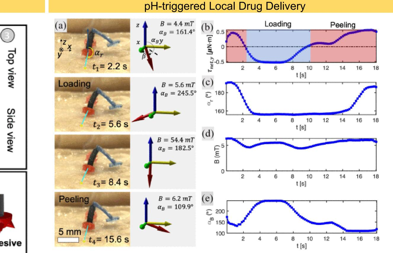
Side peeling-and-loading to attach a drug patch on soft tissues. (a) Video snapshots and magnetic fields when a robot carrying a patch on a cantilever beam and loading the patch on a soft tissue. The light blue line indicates the robot magnetic moment direction (yellow circle: end point). (b) Calculated net magnetic torque exerted on the robot. (c) The tracked robot body angle as a function of time. (d), (e). The measured external magnetic field magnitude (d) and angle (e) in the workspace.
