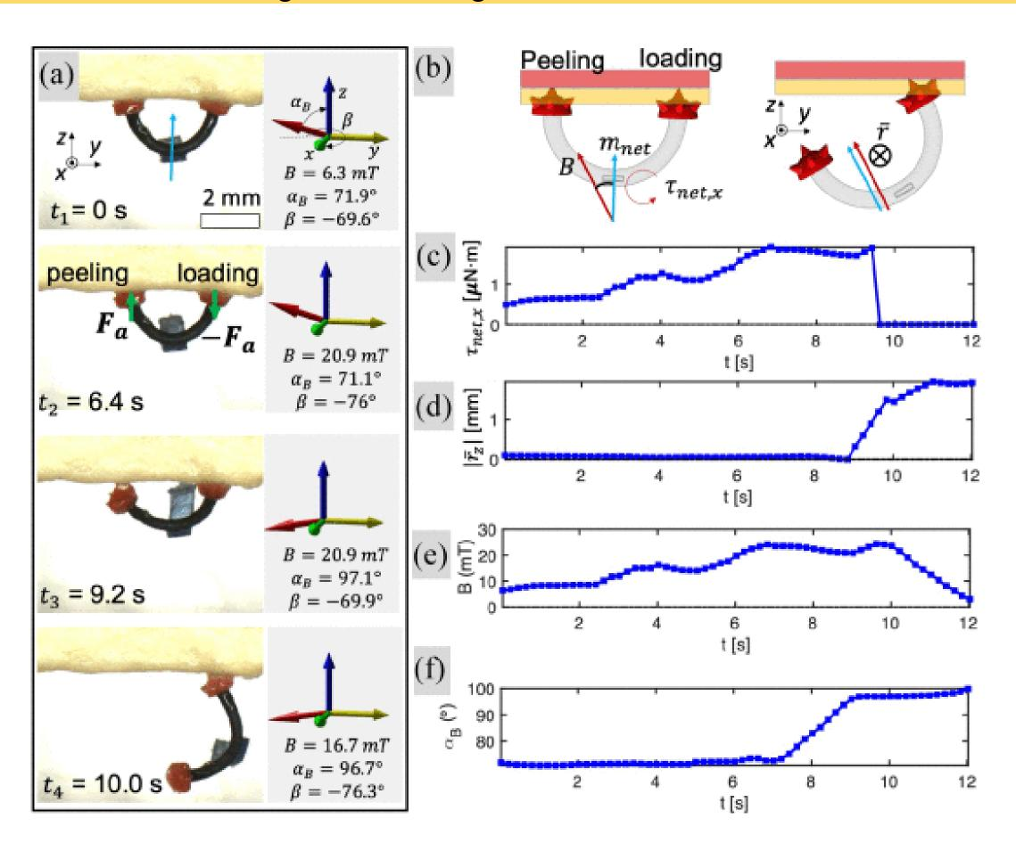
Controllable peeling-off of a robot footpad from tissue surfaces. (a) Video snapshots of a robot being peeled off from the tissue by applying an external magnetic field. (b) Schematics of the peeling process. (c) The external magnetic field for peeling and rotating. (d) Net magnetic torque exerted on the robot. (e) Applied external magnetic field magnitude. (f) The angle between the external magnetic field and the robot body symmetric axis...
