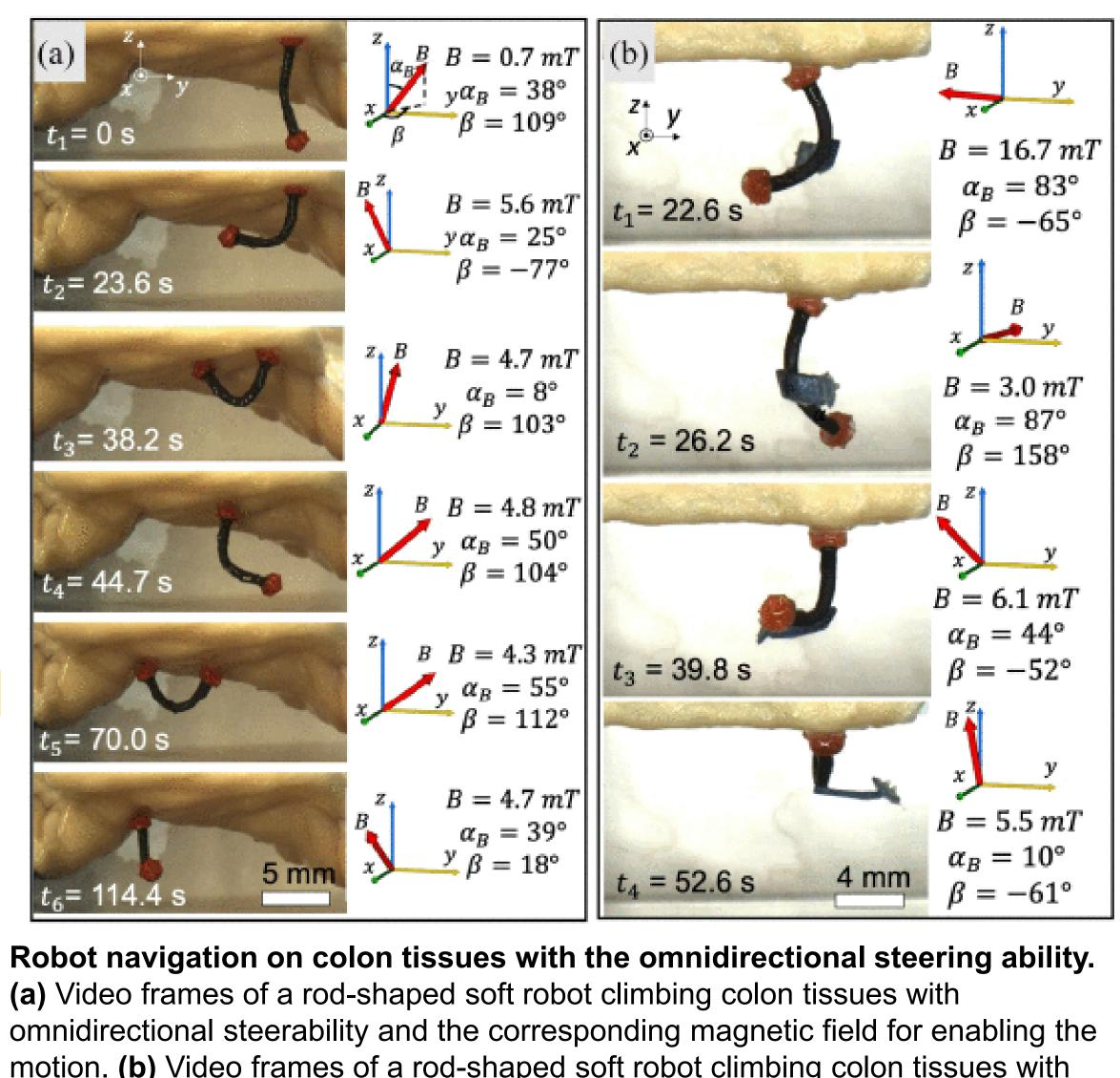
(a) Video frames of a rod-shaped soft robot climbing colon tissues with motion. (b) Video frames of a rod-shaped soft robot climbing colon tissues with omnidirectional steerability while carrying a cantilever beam for delivering a medical patch.
