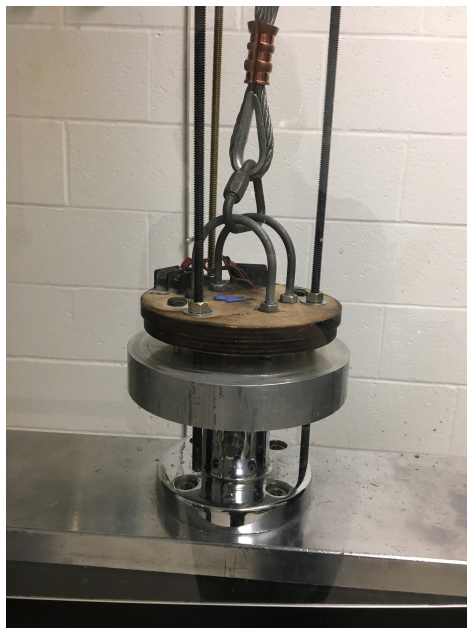
Figure 20: Wooden Bulkhead Test Set-up
