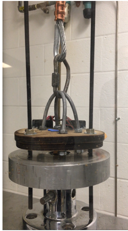
Figure 21: Wooden Bulkhead Failure Point at 2,221 Pounds
