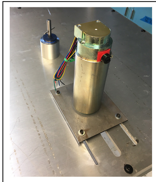
Figure 131: Picture of DC Motor Used to Simulate Aerodynamic Damping via Torque Inputs
