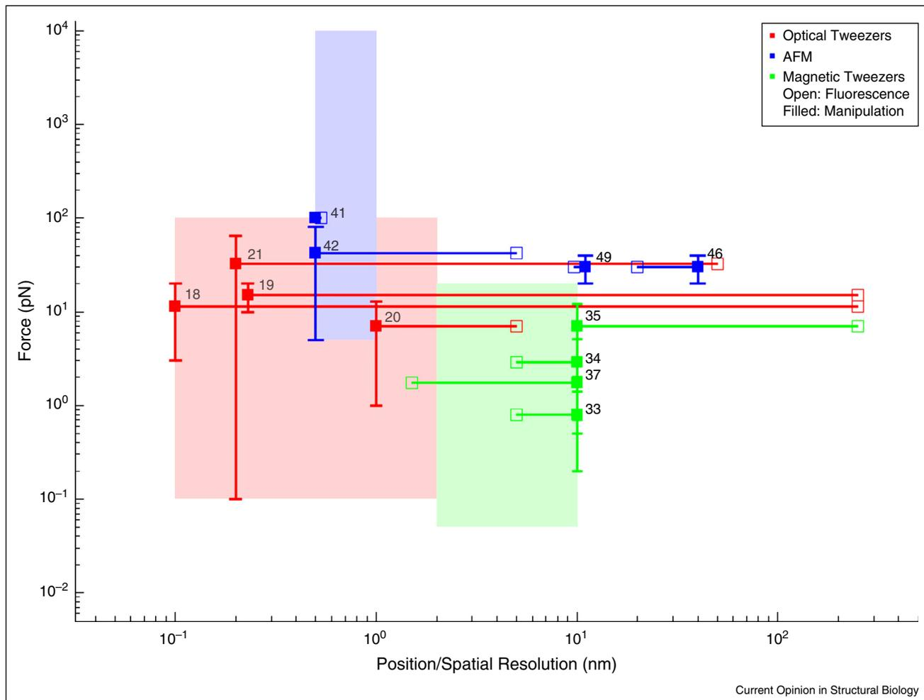
Clusters of combined methods for optical tweezers (red), AFM (blue) and magnetic tweezers (green) with fluorescence. Numbers adjacent to the squares represent the reference number in the text. Filled squares represent the position resolution for the manipulation techniques; open refers to the spatial resolution for fluorescence detection. Light colored regions are typical force ranges and spatial resolutions of the three manipulation techniques.
