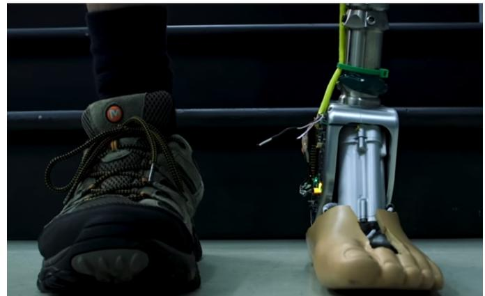
*This "smart" prosthetic ankle has a tiny motor, actuator, sensors, and chip that work together to either conform to the surface the foot is contacting or remain stationary, depending on what the user needs. (Photo: Vanderbilt University)*
