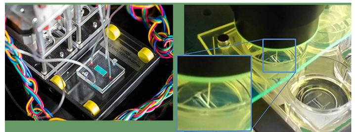
*NeuroVascular Unit and its perfusion controller, left, and the cardiac I-Wire system, right. (Photo: Vanderbilt University)*
