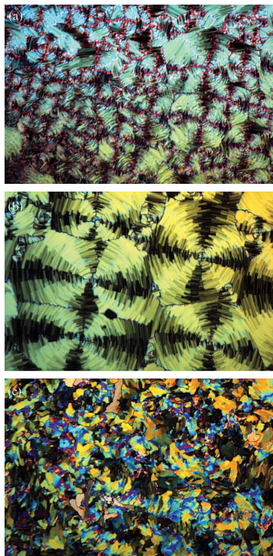
Fig. 3 Natural textures observed in polarized light for 1B in the same sample region for a) SmA phase, b) SmB phase, and c) G phase in the middle of the phase range. Magnification 60\times .
