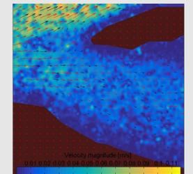
Figure 7. 0.280 ml/sec shows slower flow through the widened channel
