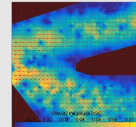
Figure 6. 0.020 ml/sec shows slightly faster flow through the widened channel
