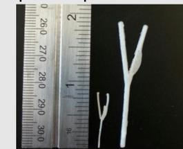
Figure 8. 0.50mm scaffold compared to 1.4mm scaffold
