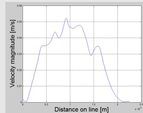
Figure 4. Graph shows velocity profile of the region denoted by the white line on figure 2. This graph shape is characteristic of fluid flow through a pipe.
