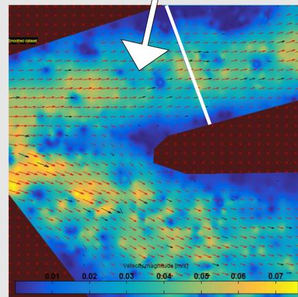
Figure 3. Velocity map given by PIVLAB analysis of device at 2.5x magnification
