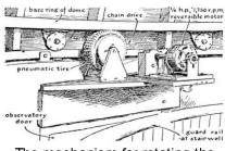
The mechanism for rotating the dome
