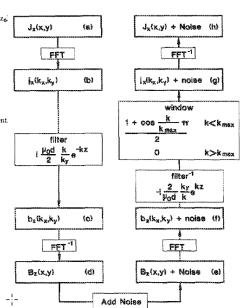
FIG. 4. Schematic diagram summarizing the forward and inverse problems. Starting with a known x component of the current density,  $J_x(x,y)$ , we calculate the z component of the magnetic field,  $B_z(x,y,z)$ , then add noise, and cross the loop cross section is Gaussian, with  $\lambda = 0.15$  mm. calculate an image of the current density from the noisy magnetic field.
