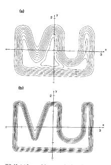
IG. 12. (a) Image of the current density, calculated from the noisy magsetic field in Fig. 1: z = 1.0 mm,  $k_{\text{max}} = 10 \text{ mm}^{-1}$ , noise = 0.5 pT, a = 0.35nm, and MSD = 0.40. (b) Current density used to calculate the magnetic ield in Fig. 1. The loop carries 1  $\mu$ A of current, and the current profile
