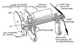
Readout mechanism for monitoring declination; numbers refer to gear teeth
