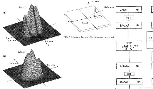
FIG. 1. Two views of simulated magnetometer data. The magnetometer coil, radius 0.35 mm, detected the normal component of the magnetic field, B,, over a plane 1 mm above a two-dimensional current source. The magnetometer signal has an amplitude of 190 pT and contains 0.5 pT of noise. Our goal is to reconstruct an image of the current distribution that produced this magnetic field.
