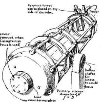
Tube of the telescope
