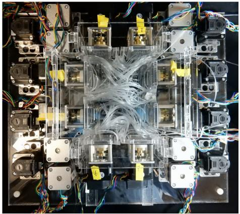
Use time-division multiplexing to individually formulate, deliver, and remove custom media cocktails to each well of a 96-well plate to simulate PK profiles.
