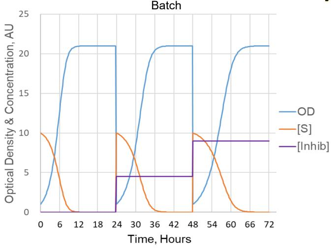
Three serial-batch measurements of yeast growth with differing inhibitor concentrations.
