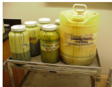
Improper Hazardous Waste Storage. No VEHS labels, no secondary containment, no segregation, and containers are covered with residue.
