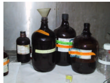
Improper Hazardous Waste Storage. No VEHS labels, no secondary containment, and container not sealed properly (open funnel).
