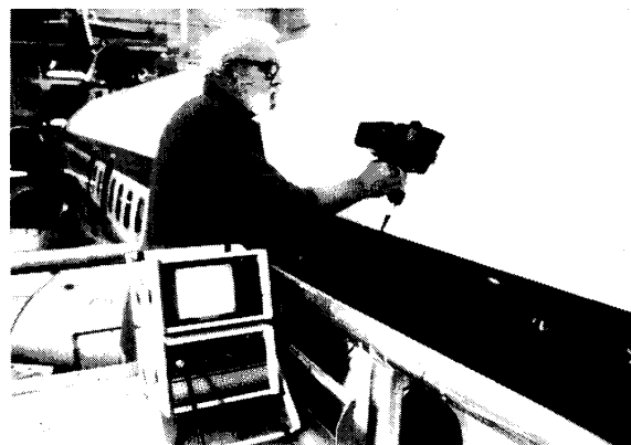
Fig. 48. The PRI magneto-optical inspection (MOI) system being used to find fatigue cracks in an airplane fuselage. (Courtesy of Gerald Fitzpatrick of PRI)
