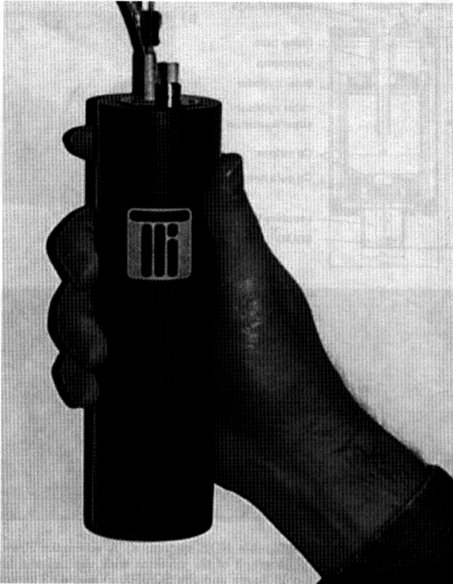
Figure 22. A hand-sized liquid nitrogen dewar developed by Tristan Technologies, Inc. that has a single high- T_c SQUID in it. It has an 8-hour hold time when vertical and a 4-hour hold time in any other orientation. (Courtesy of Robert Fagaly, Tristan Technologies, Inc.)
