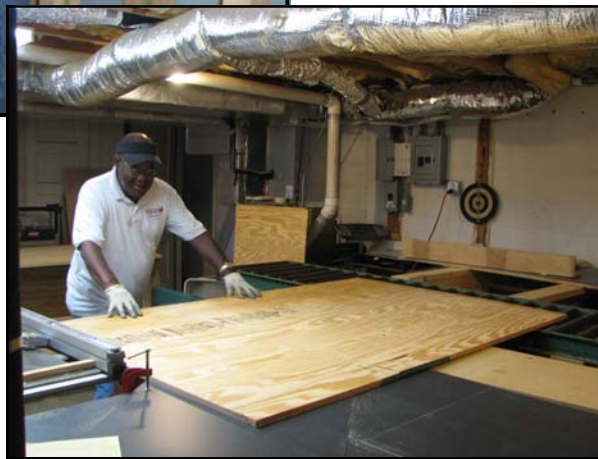
Cutting plywood for athletic lockers
