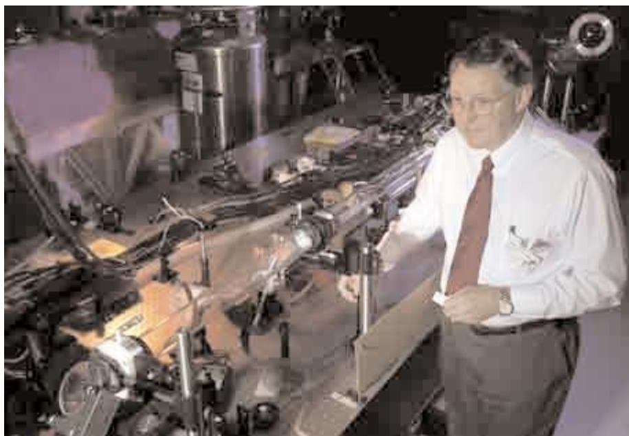
▲ Frank Carroll, MD, stands by the tabletop terawatt laser with a test paper. He believes the new monochromatic X-ray machine will revolutionize diagnostic imaging.
