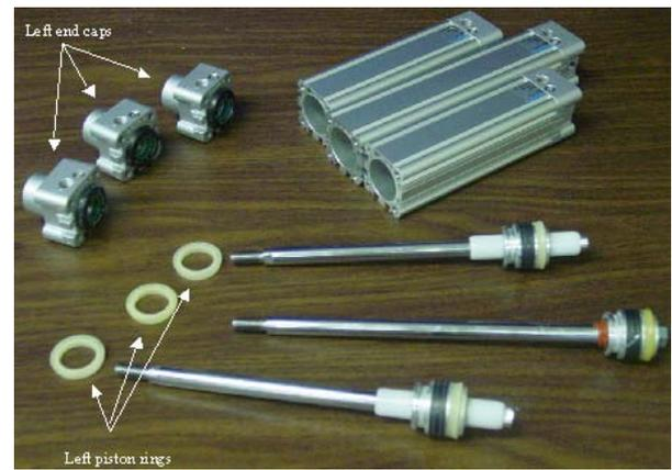
Figure 5: Removal of left piston seals and end caps.
