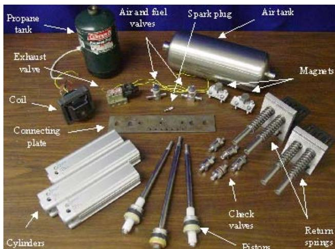
Figure 4: Exploded view of FPC hardware.
