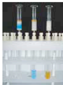
Figure 1. A Fluorous Solid-Phase Extraction of Organic (Blue) and Fluorous (Orange) Dyes over FluoroFlash ® Silica Gel.
