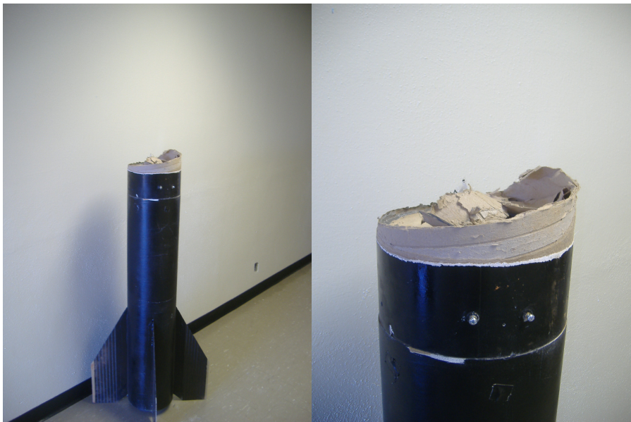
Figure 2a,b showing the rupture at the midsection that destroyed the rocket at 2500 ft altitude.
