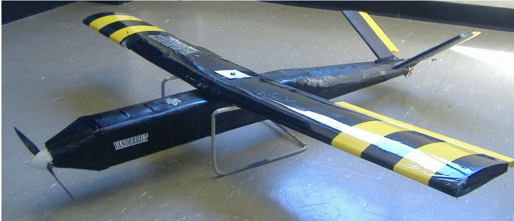
Fig. 1a2: The actual Reconnaissance UAV that was hand-built from CAD drawings
